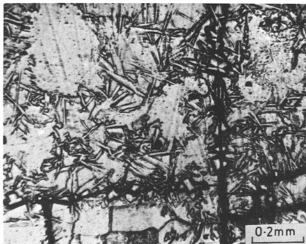
Fig. 10. Irregularly oriented martensitic laths within galena. The squarish to rectangular platelets are concentrated along grain boundaries. Etched with thiourea + HCl. Reflected ppl, in air
