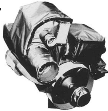
Fig. 4. Remote sensing capability of Voyager science instruments. Insert shows scan platform optical instruments and thermal blankets.
