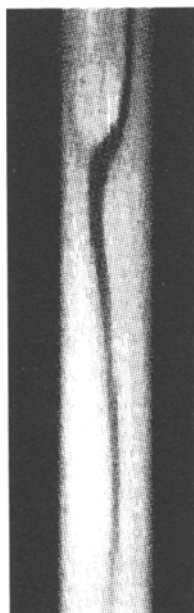
Fig. 18. Azimuthal instabilities leave a wavy strip of Fluid 1 in the narrow side
