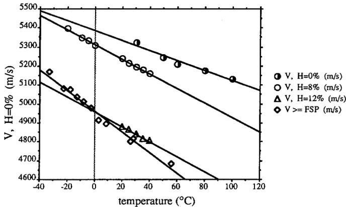
Fig. 4. Influence of temperature on the ultrasound wave propagation speed,  $V_m$ , for different moisture contents
