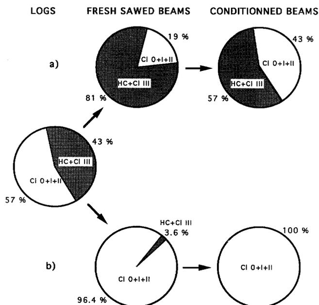
**Fig. 6 a and b.** Ultrasound grading applied to logs. Evolution of the grading at the different levels of transformation from log to conditioned beams. a) weakest beams; b) strongest beams
