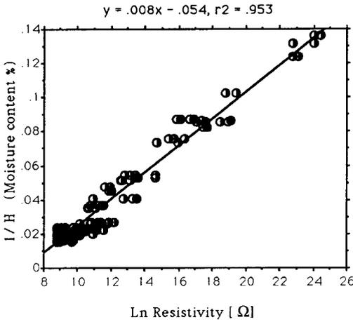
**Fig. 2.** Relationship between wood logarithmic resistivity and the inverse of moisture content,  $H_i$ , for a range of  $H = 6\%$  to  $H = 100\%$
