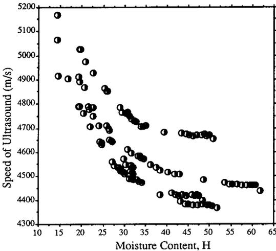
**Fig. 3.** Influence of moisture content on the ultrasound wave propagation speed in the range of  $H = 6\%$  to  $H = 70\%$  for a sample of 30/30 mm cross section
