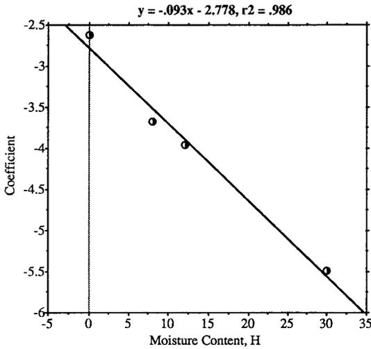
**Fig. 5.** Effect of moisture content on the slope of the temperature versus propagation speed relationship observed in Fig. 4
