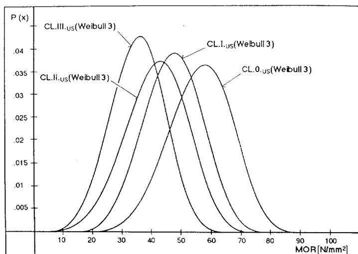
**Fig. 1.** Probability density functions of the modulus of rupture, MoR, for different ultrasound graded classes, including a new high performance class, class 0. The distributions are three parameter Weibull model based. (Sandoz 1991)
