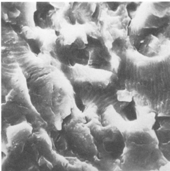
Figure 10. Striations in 683 alloy; (a) air, (b) water vapor. The crack growth direction is upwards.
