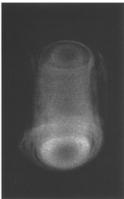
Fig. 4. Photograph of vortex ring generated with setting s1f. Re = 400
