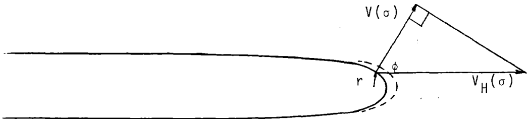
Figure 4: Crack extension due to stress corrosion.
