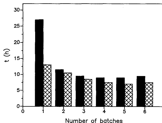
Fig. 3. Semicontinuous degradation of phenol (1 g/l) by the activated carbon and sintered glass systems. Activated carbon system, \blacksquare ; sintered glass system, \blacksquare
