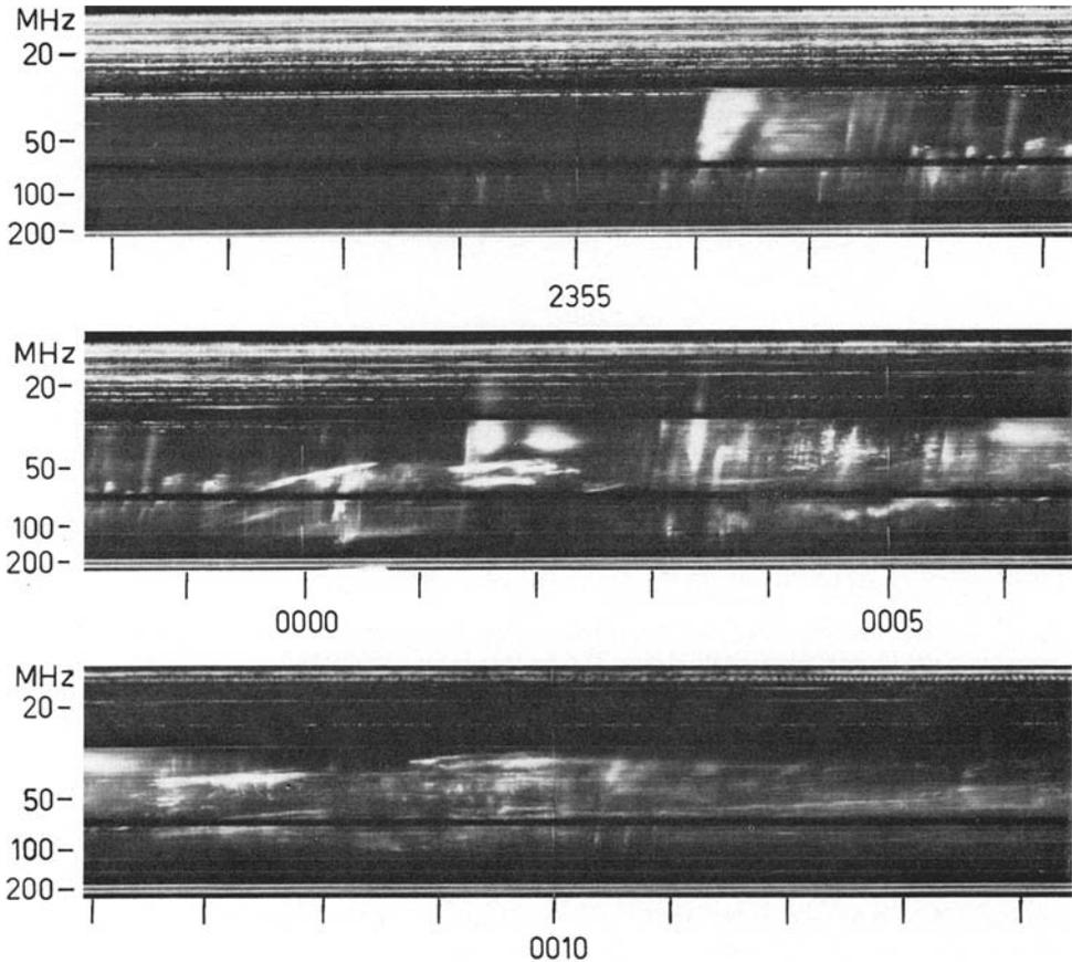
Fig. 1. Dynamic spectrum of the complex type II bursts on 1968, October 23-24.
