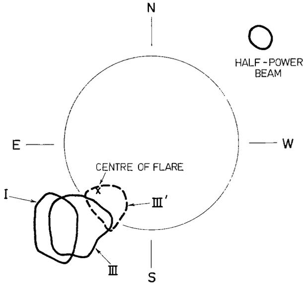
Fig. 2. 80 MHz sources of the type I storm and the type III bursts. The outlines represent half-power levels. Source I: the preceding type I storm. The contour is for  $23^{\text{h}}53^{\text{m}}$ . Source III: a type III burst at  $23^{\text{h}}54^{\text{m}}07^{\text{s}}$ . Source III': a burst of peculiar type III at  $00^{\text{h}}00^{\text{m}}16^{\text{s}}$ . *N* in this and the Figures 3 to 5 indicates the north point of the Sun.
