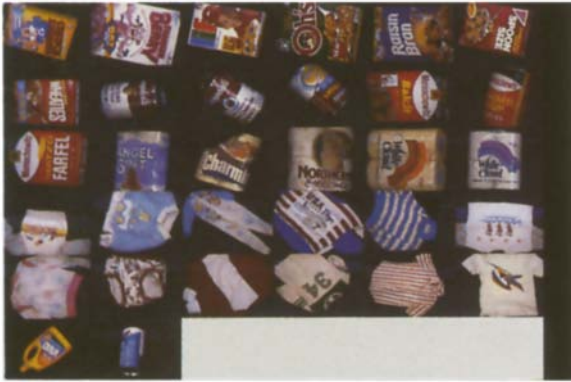
Fig. 5. The unknown objects. Each is identified with the model color histogram that best matches its own color histogram. Compared to the models the unknown objects are translated (Ajax), rotated about various axes (Frankenberry, Ajax) scaled (USA Flyer), occluded (Charmin), partly outside of the field of view (red, white striped shirt), and deformed (Mickey Mouse underwear).
