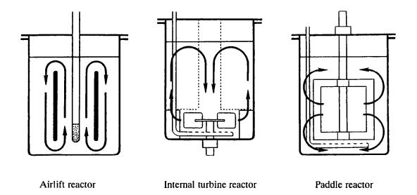
Fig. 1 Three types of reactors used in culture of embryogenic tissues. Arrows showed the streams of media in the reactors.
