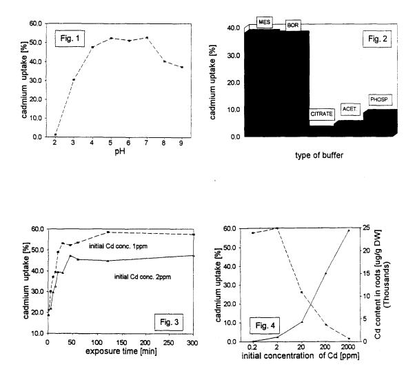
Fig.1: Dependence of  $Cd^{2+}$  uptake on pH of test solution , (initial  $Cd^{2+}$  concentration 2ppm)
