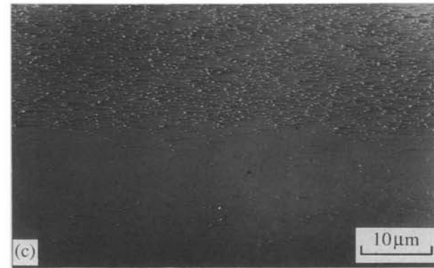
Figure 8 The new bone-Ti-6Al-4V interface near the centre of the edge face of the implant (arrow, Fig. 7d) showing a thin layer of fibrous membrane together with an artificial gap interposed 6 weeks post-implantation. (a) Image from SEI-SEM, (b) image from BEI-SEM, and (c) WDS X-ray mapping of Ca trace. N, new bone; M, bone marrow; F, fibrous membrane; T, Ti alloy; G, artificial gap.
