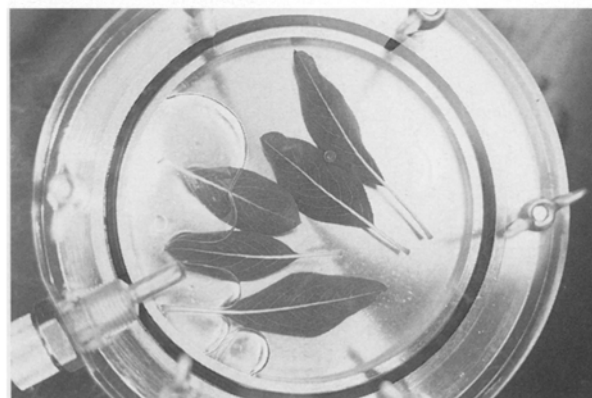
Fig. 1. Infiltration chamber with Pyrus amygdaliformis leaves at (A) beginning of infiltration and (B) at 90% infiltration.
