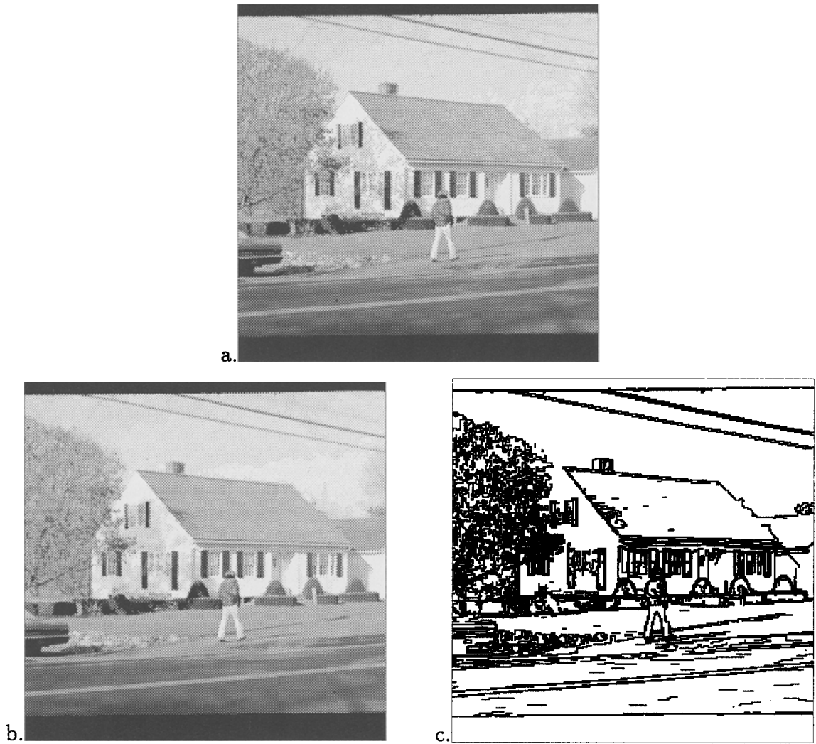
Fig. 5. a. An 8-bit image of 256 \times 256 pixels. b. The smoothed image for final \mu = 0.7 , \gamma_{ij} = 60 , and 500 iterations. c. The corresponding line process.
