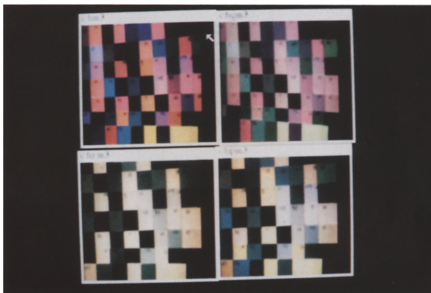
Color Figure 11. Outputs of Crule for the third Mondriaan derived from images under (clockwise, from top left) white, green, purple, and red lights. Crule is not performing very well on these images, because they do not contain a wide range of colors.
