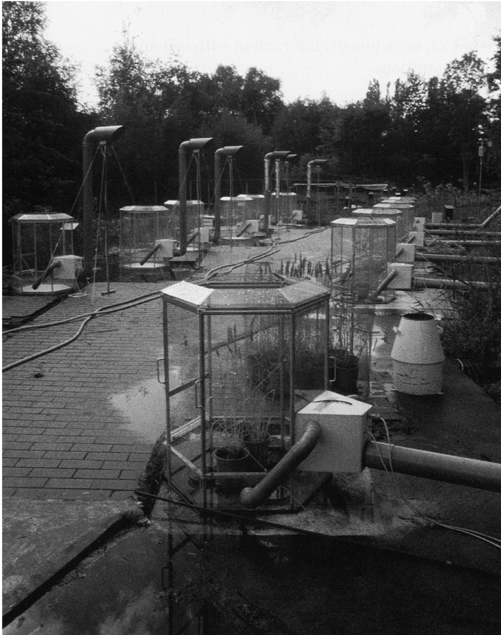
Open Top Chambers used for assessment of the response of wheat ( C_3 ) and maize ( C_4 ) plants to atmospheric carbon dioxide enrichment. (Photograph J. Rozema).
