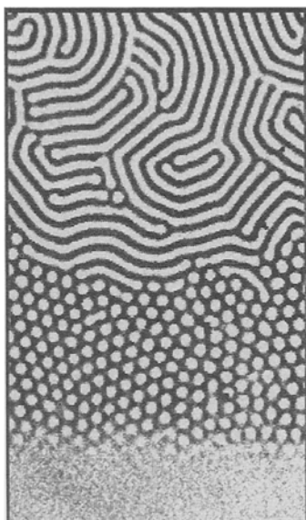
Fig. 4. Monolayer patterns in a bevelled disc. (Circular faces making an angle of 4 degrees, bottom width 1.9 mm, top width 3.4 mm). View of a bottom portion of the disc. From bottom to top: uniform state \rightarrow hexagons of spots \rightarrow stripes. Experimental conditions; temperature = 6°C, residence time in reservoirs = 6 min, [starch] = 2.1 g/l of gel, [I^-]_I = [I^-]_{II} = 2 \times 10^{-3} M, [\text{ClO}_2^-]_{II} = 5 \times 10^{-2} M, [\text{MA}]_I = 1.3 \times 10^{-2} M.
