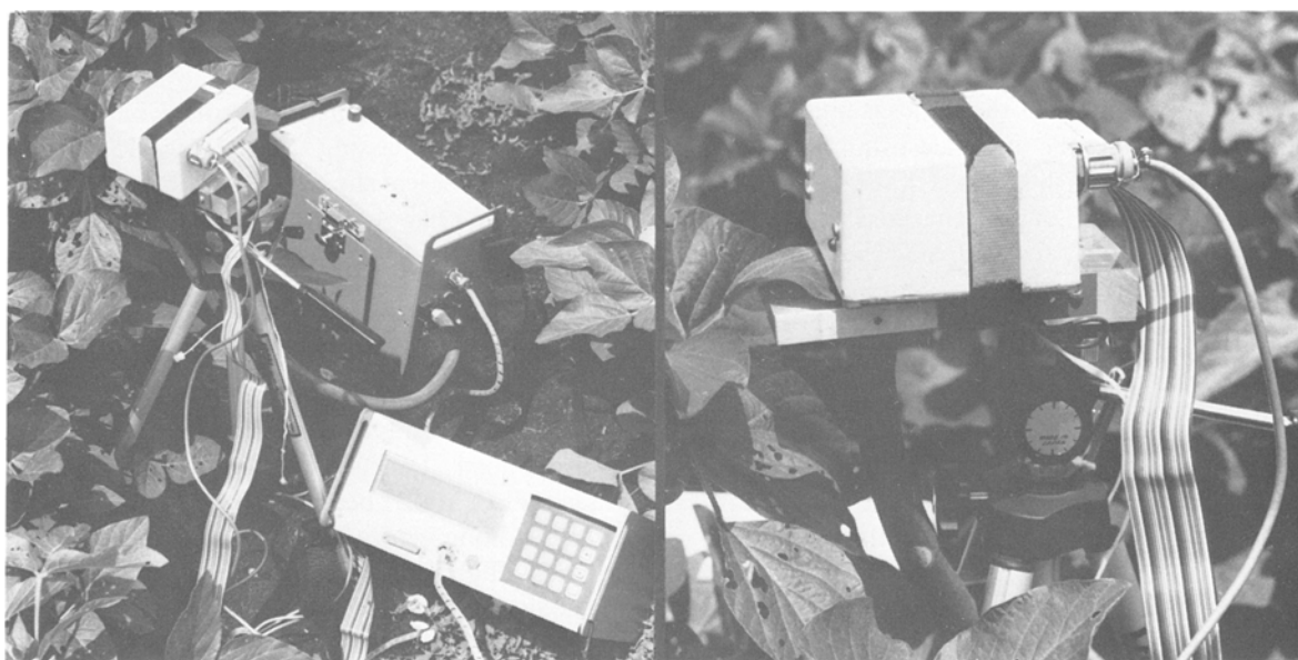
Fig. 1. Photographs of the portable double-flash spectrophotometer. Left: The instrument consists of three portable boxes. The first of these contains the two flash lamps, one for the actinic flash, another for the measuring flash, high voltage power supplies to run them, and optics leading to a specially constructed fiber optics network. The fiber optics bundle carries the light to the leaf chamber which is mounted on the second box. This box contains the photodiode detectors and blocking filters, and the analog electronics. The third box contains a microcomputer to run the experiments and to collect, store, manipulate and display data. Right: Detail showing leaf clamp/detector holding a leaf. The total weight of the instrument, including batteries, is about 17 Kg.
