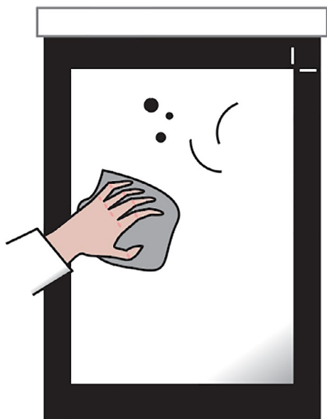
Figure 1-16. An illustration of a person cleaning the flatbed scanner glass and removing smudges and dust before use
