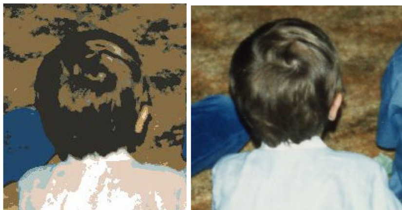
Figure 1-35. Choosing a color mode of color smoothing for this print from the scanner dialog box is not the best choice; in this case, it would be better to use 24-bit color
