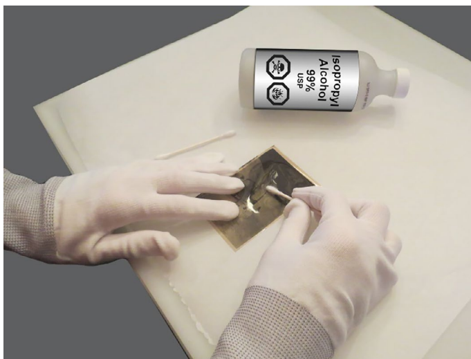
Figure 1-4. Carefully cleaning the shiny side of a black and white negative with gloves and a cotton swab dipped in Isopropyl Alcohol
