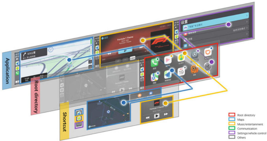
Fig. 8.2 Three hierarchy layers of the Apple CarPlay interaction structure
