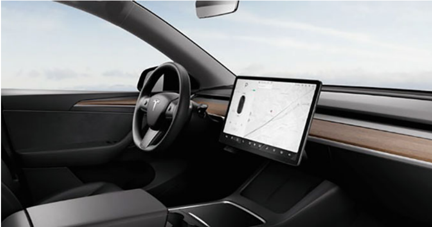
Fig. 5.12 Tesla Model 3 (2017) without central console buttons and instrument cluster display (Source Tesla, Inc.)
