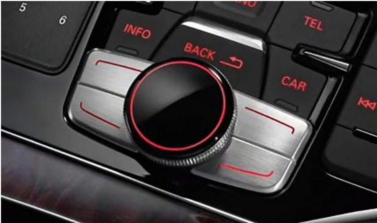
Fig. 3.2 MMI knob of the Audi A8 (2011 model), which was later removed in the new generation (Source Audi AG)
