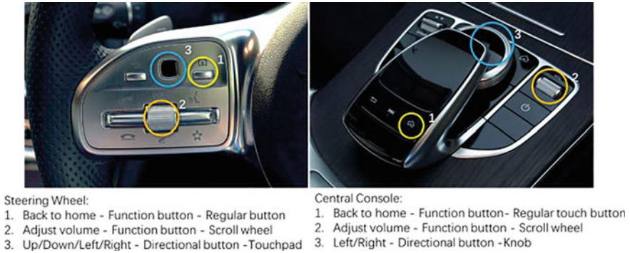
Fig. 6.7 Function and directional buttons on the steering wheel and central console area of the Mercedes-Benz C-Class (2019) (Source The Mercedes-Benz Group)
