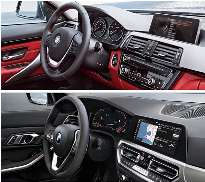
Fig. 5.14 Central information display of the BMW 3 Series (2019, bottom panel), which is positioned closer to the driver than in its predecessor (top panel) (Source The BMW Group)
