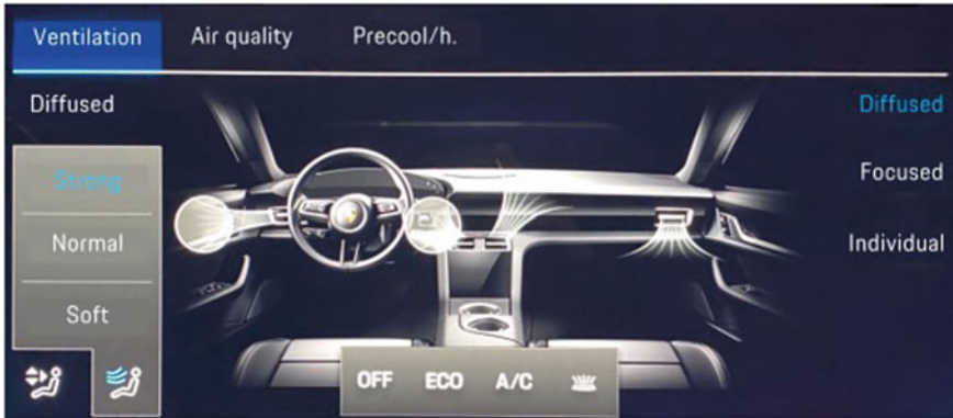
Fig. 8.12 Climate control interface of Porsche Taycan (2020), wherein users can adjust the airflow direction by dragging the circles on the two left-side air vents with fingers, translated from Chinese language
