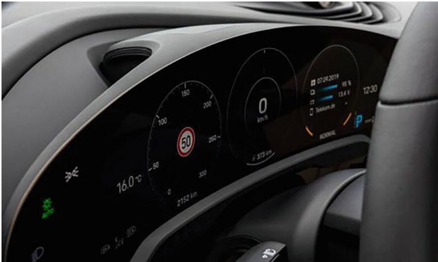
Fig. 5.10 Concave curved instrument cluster display of the Porsche Taycan (2020) (Source Porsche AG)
