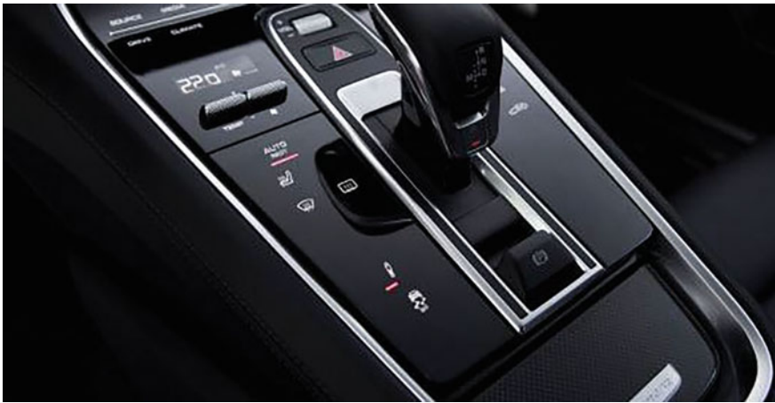
Fig. 5.17 Touch-sensitive buttons with vibration feedback in the Porsche Panamera (2017) (Source Porsche AG)
