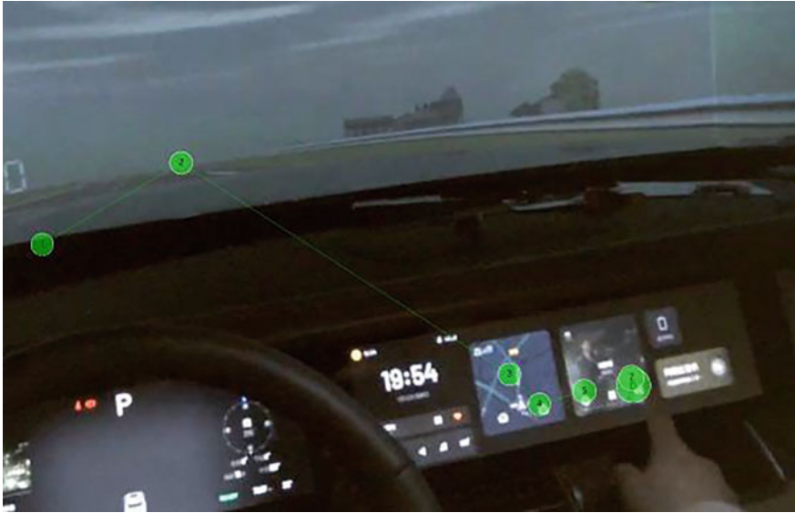
Fig. 7.4 Fixation distribution when using the touchscreen to switch to the next music track in the Li Auto One
