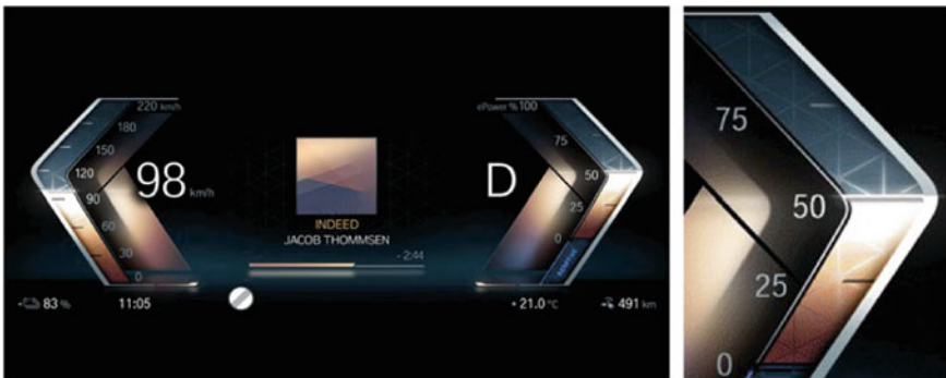
Fig. 11.6 Instrument display interface and partial magnification of the BMW's iDrive 8 system (2021) (Source BMW Group)
