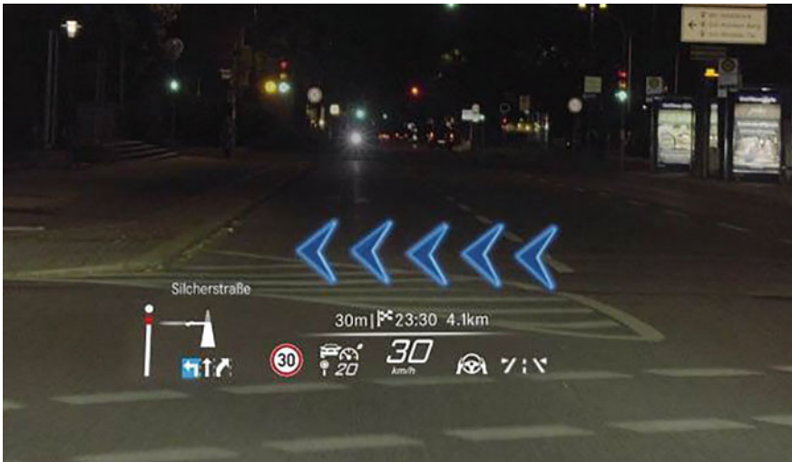
Fig. 5.5 AR navigation on the HUD of the Mercedes-Benz S-Class (2020) (Source The Mercedes-Benz Group)
