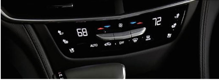
Fig. 5.16 Pressure-sensitive buttons in the Cadillac CT6 (2017) (Source General Motors Company)
