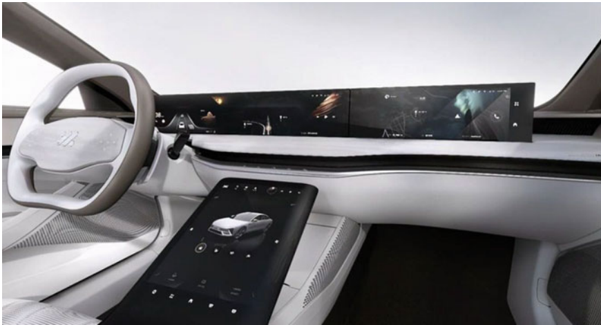
Fig. 10.8 Retractable instrument cluster display, central information display, front passenger display, and lower control display in IM L7 (2022) (Source IM Motors)
