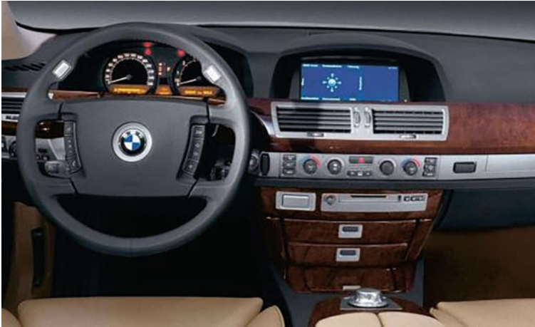
Fig. 1.3 iDrive system with a combination of knobs and a non-touch central screen in the BMW 7-Series (2001) (Source BMW Group)
