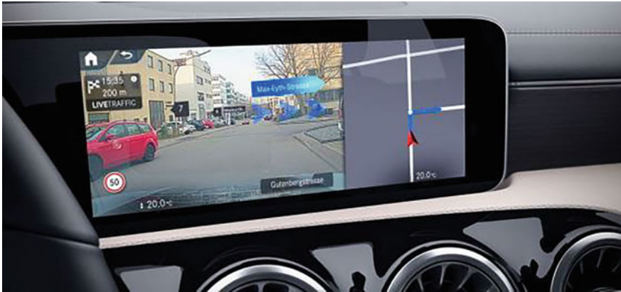
Fig. 5.4 AR navigation on the central information display of the Mercedes-Benz A-Class (2019) (Source The Mercedes-Benz Group)
