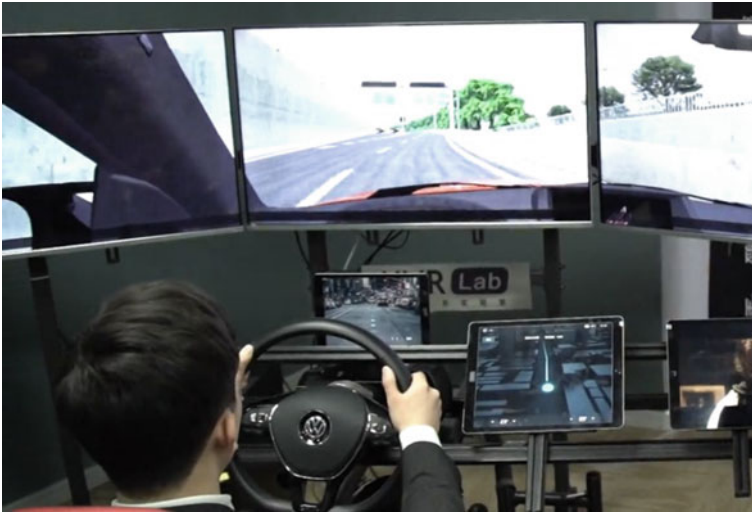
Fig. 12.3 Rapid concept prototype seating buck
