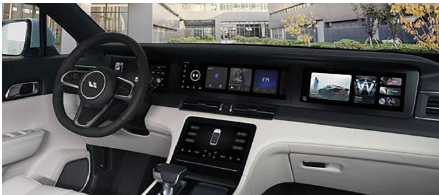
Fig. 5.15 Central information, instrument cluster, and front passenger display of the Li Auto One (2020), positioned on the same plane (Source Li Auto, Inc.)
