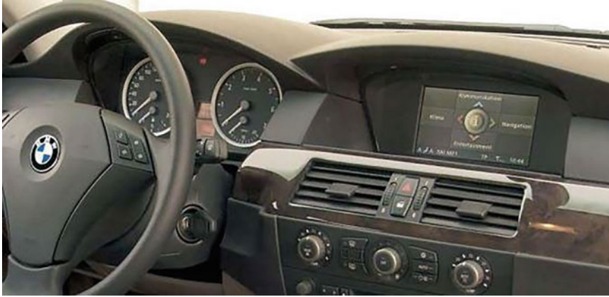
Fig. 5.9 Downward-sloping transparent cover outside the central information display and instrument cluster display of the BMW 5-Series (2004) (Source The BMW Group)
