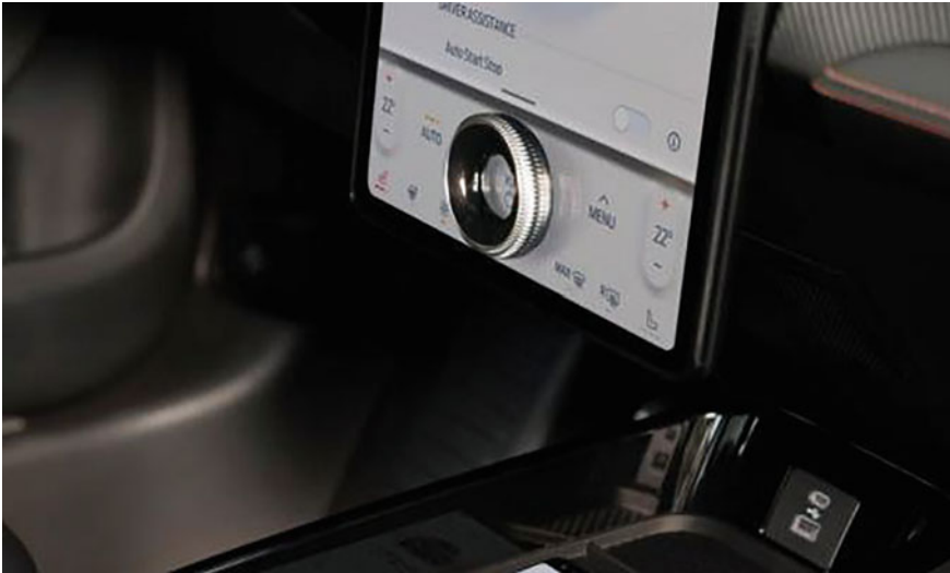
Fig. 5.18 Physical knob on the central information display of the Ford Mustang Mach-E (2021) (Source Ford Motor Company)
