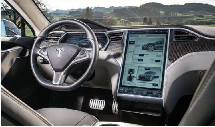
Fig. 1.4 Tesla Model S (2012) with a large 17-inch central information display ( Source Tesla, Inc.)
