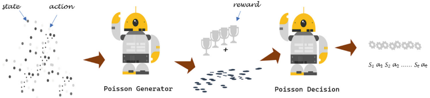
Fig. 1. Planning with Poisson Decision. Given the current state and action, Poisson Decision uses Classifier-Guidance generate a sequence of future states and action, It then extract the best trajectory by modifying the means \mu of the reverse process according
