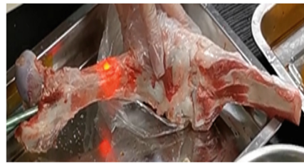
Fig. 2. Left: A schematic plot of how iMET reveals the location of a distal screw hole. Right: a pig bone phantom study that showed the red light spot projected on the bone surface that was emitted from the iMET.
