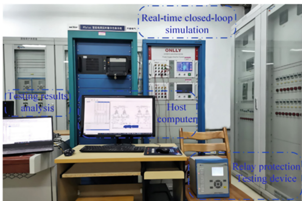
Fig. 1. RT-plus real-time digital simulation test platform
