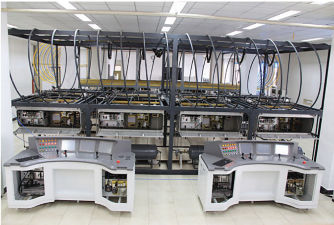
Fig.1. Urban rail vehicle braking system test platform
