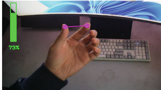
Fig. 8. Image demonstrating media volume controlled by hand gestures
