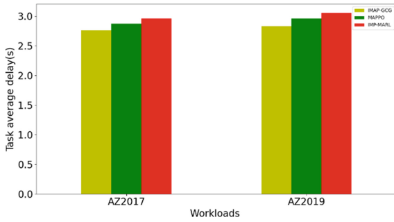
Fig. 5. Comparison of task average delay on different workloads
