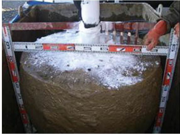
Fig. 6 Excavated frozen soil
