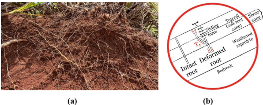
Fig. 1 a Exposed root-soil zone after shallow slope failure, b sketch showing root tensile strength activated from sliding forces in root-soil zone
