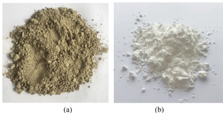
Fig. 1 Materials used in this study: a the commercial clayey soil, b the \text{MgCO}_3 powder
