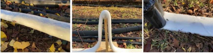
Fig. 18 Frosted pipe from each case (left–case 1, center–case 2, right–case 3)
