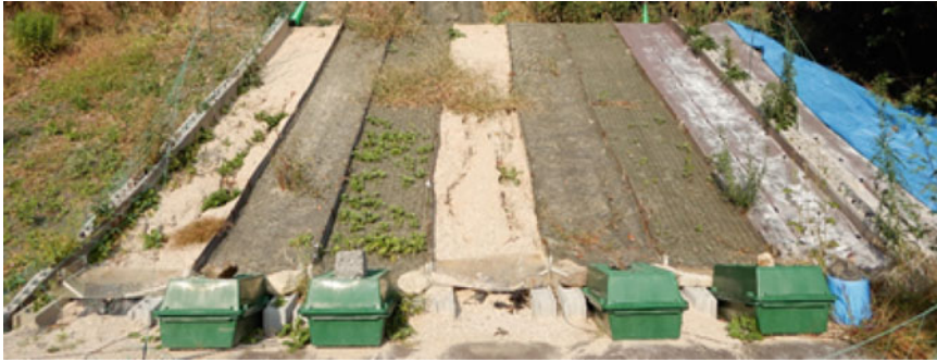
Unprotected soil_1 Erosion control mat A_1 BSC mat_1 Unprotected soil_2 Erosion control mat A_2 BSC mat_2
