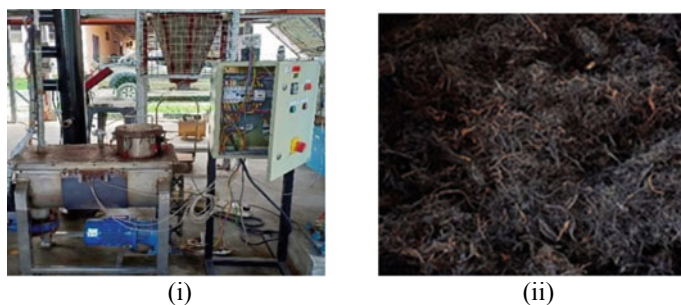
Fig. 1 (i) Rotary carbonizer. (ii) Carbonized EFB fibers
