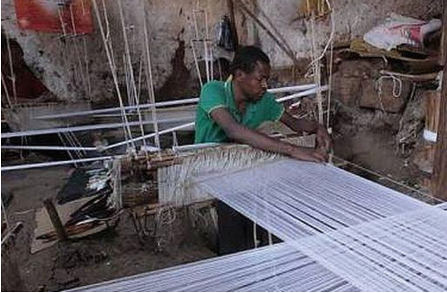
Fig. 6 Pit ground loom (Photograph by author)
