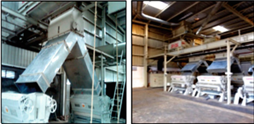
Fig. 18 Twin auto regulator individual gin feeding conveyor system. Source [40]
