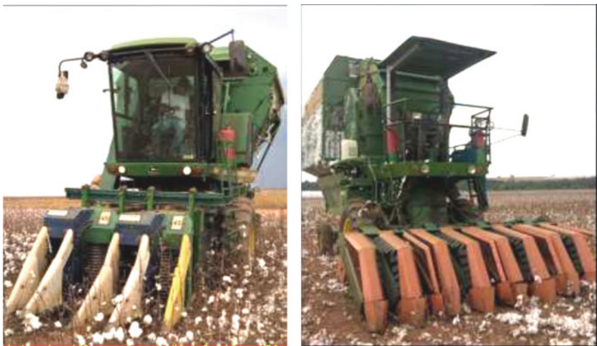
Fig. 1 John Deere model 9930 Pro-12 VRS (variable row spacing) cotton picker (left). John Deere model 9960 brush-type cotton stripper with a view of the coupled field cleaner (right)
