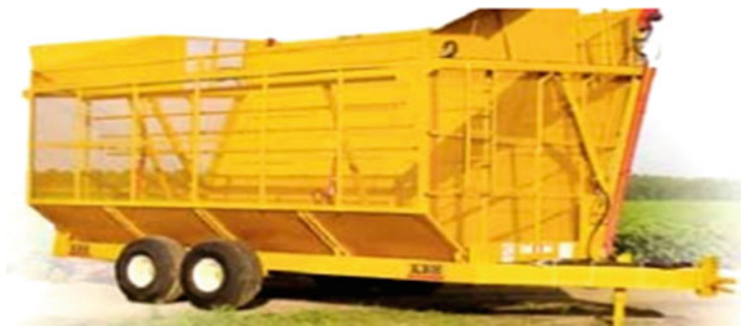
Fig. 5 The boll buggy used to transport harvested cotton between the harvester operating in the field and the module builder located at the edge of the field (Photo courtesy of KBH, Inc.)
