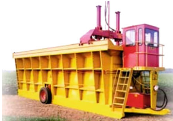
Fig. 4 A modern module builder with cab for operator comfort and hydraulic drive system. A tractor provides PTO power to drive the hydraulic pump and drawbar power to move the builder (Photo courtesy of KBH, Inc.)
