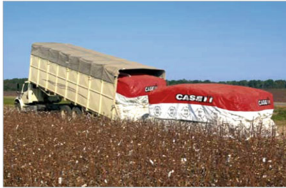
Fig. 7 Two case IH half-length modules staged together and being loaded into a module truck. Source [40, 41]
