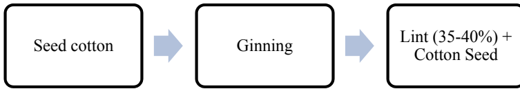
Fig. 2 Simplified ginning process. Source Authors
