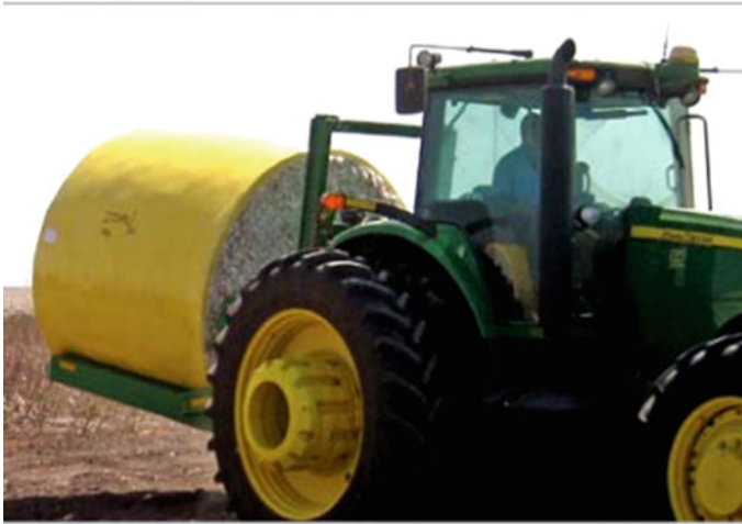
Fig. 9 Carrying a round module with a three-point hitch attachment. The module is being staged for transport to the gin. Source [40, 41]
