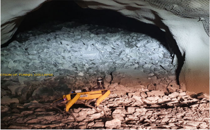
Fig. 1.5 Robot dog inspecting a roof collapse site in a mine (courtesy LKAB)
