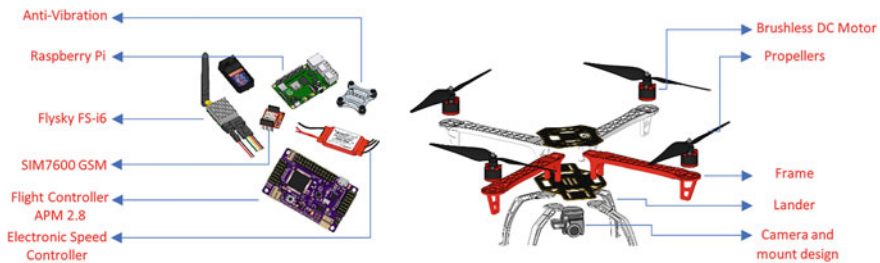
Fig. 2 Complete drone parts and shows alignment of motors, propellers, lander, and camera on frame
