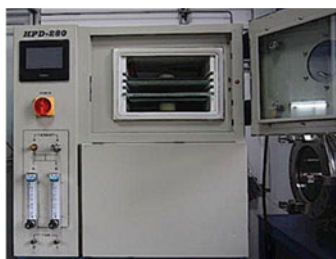
(a) Physical view of the glow discharge modified cavity
