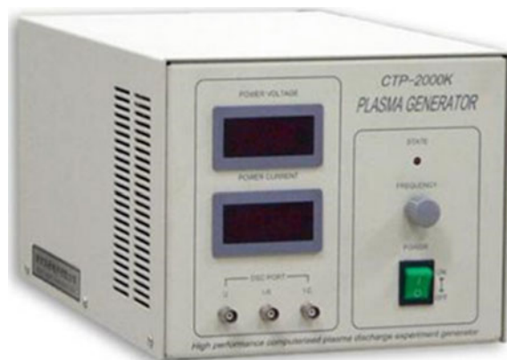
Fig. 5 Actual photograph of high frequency high voltage power supply
