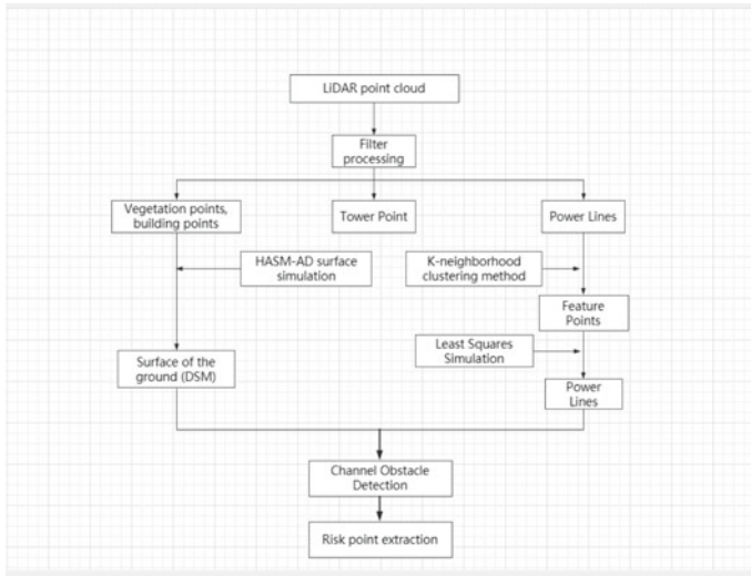
Fig. 2 Basic idea of safe distance detection of transmission lines in the airborne LiDAR system
