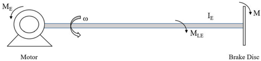
Fig. 2 Force analysis of electrical inertia simulation solution
