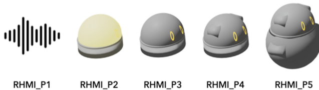
Fig. 1. RHMI prototypes (RHMI-P) that are used for the Study 1: RHMI-P1: sound-only, RHMI-P2: illuminated dome, RHMI-P3: dome with eyes, RHMI-P4: dome with eyes and ears, RHMI-P5: full body
