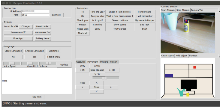
Fig. 4. GUI for operating the robot using the Wizard-of-Oz method. We control the language (left-middle), speaking (top-middle), and head movements (bottom-middle), and display the current scene on the tablet when needed (bottom-right). We can also watch the scene using the robot's head camera (top-right).
