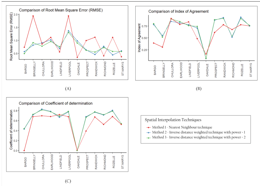
Fig. 5. Comparison of the performance of Nearest Neighbour interpolation, Inverse distance weighted interpolation with power = 1 and Inverse distance weighted interpolation with power = 2 at each site. (A) Based on Root Mean Square Error (RMSE) (B) Based on Index of Agreement (d) (C) Based on Coefficient of determination ( R^2 )
