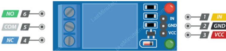
Fig. 9 5-V 1 channel Arduino relay module
