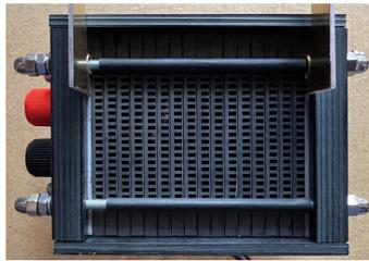
Fig. 1. Open-cathode stack
