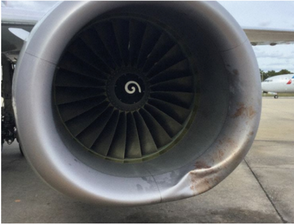
Fig. 5. Aero-engine bird strike
