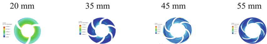
Fig. 4. Relative flow angle of each plane when axial length of the centrifugal impeller is 25 mm.
