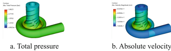
Fig. 2. Total pressure and absolute velocity of the preliminary design
