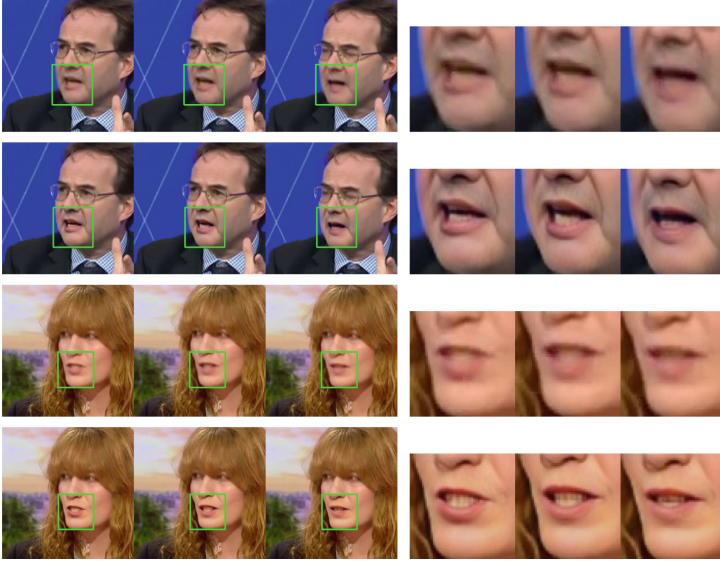
Fig. 5. Visualization results in side-faced speaker. The first and third rows are the original talking face-generated frames, and the second and fourth rows show the results of the dental restoration applied with our method. It can be clearly seen that our model produces both sharpness and color teeth details in a side-faced speaker, demonstrating the effectiveness and robustness of our method.
