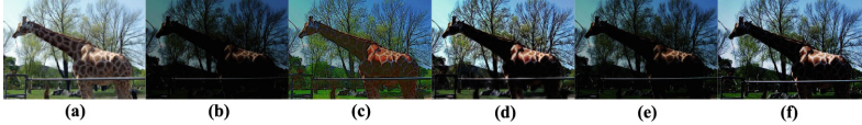
Fig. 1. Visual artifacts introduced using some recent low-light enhancement methods, where (a) is the ground-truth image, (b) is the low-light image, and (c)–(f) are the results of RetinexNet [22], KinD [26], DALE [9] and Zero-DCE++ [12], respectively.
