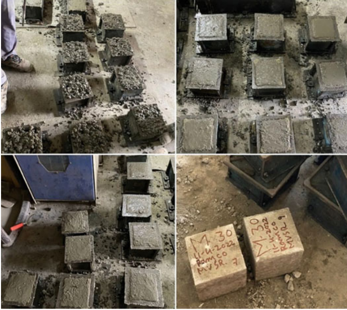
Fig. 4 Concrete cubes being cast for M30 grade
