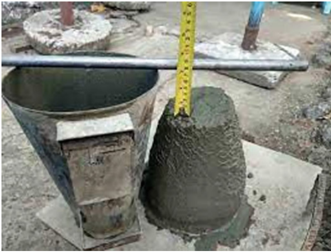
Fig. 1 Concrete slump test for workability
