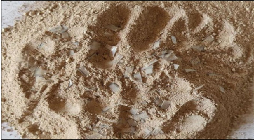
Fig. 2 Soil sample mixed with waste plastic strips
