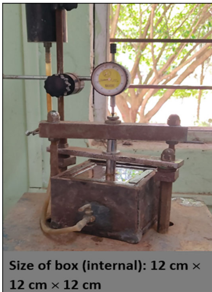
Fig. 3 Laboratory-fabricated 3D consolidation apparatus
