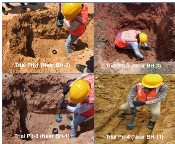
Fig. 5 Field density using the core cutter method
