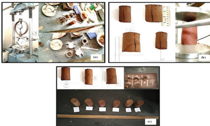
Fig. 4 Unconfined compressive strength test setup. a Instrumentation setup b, c Soil sample after deformation
