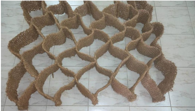
Fig. 2 Coir geocell used for the study
