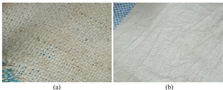
Fig. 3 Geotextiles materials, a jute textile and b polypropylene (PP) geotextile
