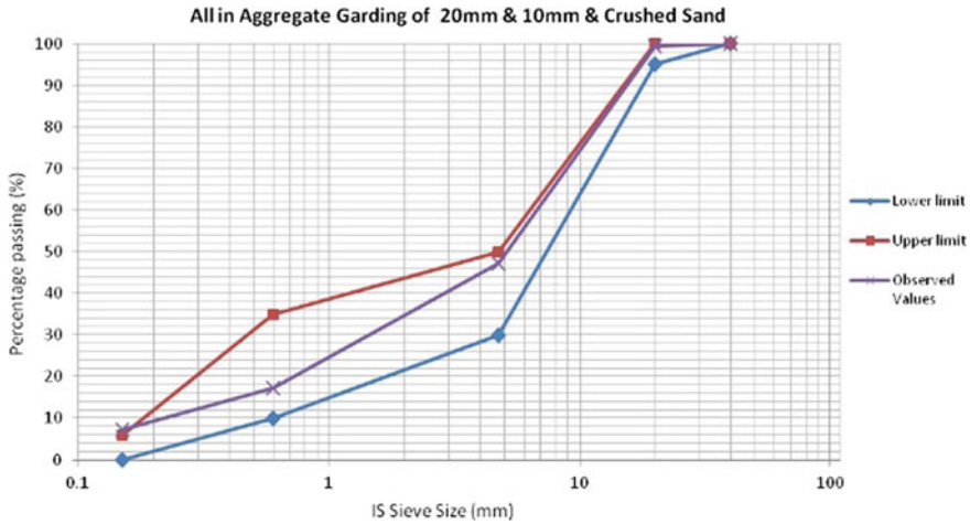
Fig. 3 All-in aggregate gradation
