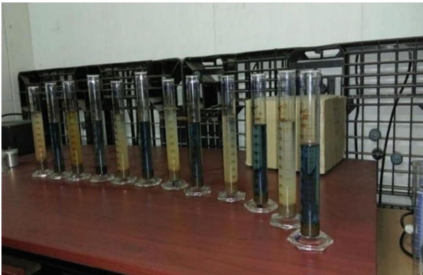
Fig. 2 Free swell index of different soil samples
