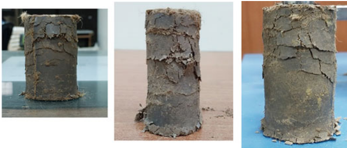
Fig. 10 From left to right, images showing comparison of jute fibre at 2, 2.5 and 3% fibre content
