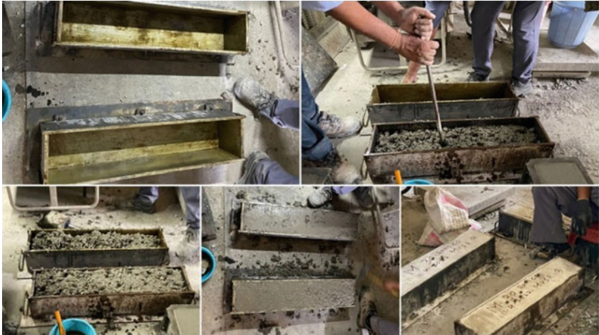
Fig. 5 Concrete beams being cast for M30 grade
