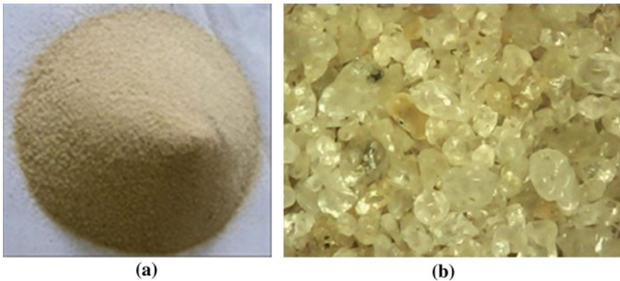
Fig. 1 a Coastal sand and b digital microscope image
