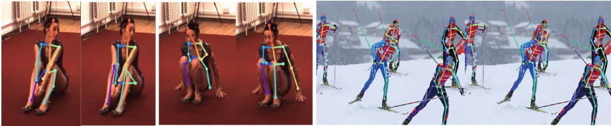
Fig. 4. Comparisons of introducing local-space attention (right) or not (left) under challenging circumstances like occlusion and overlapping multi-person.
