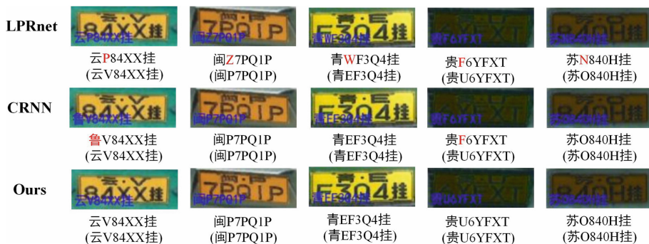
Fig. 5. The figure shows the recognition results of different algorithms on two-way license plates. The words in parentheses are the ground truth.
