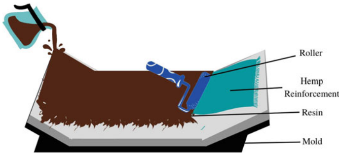
Fig. 3 The schematic diagram showing hand lay-up technique
