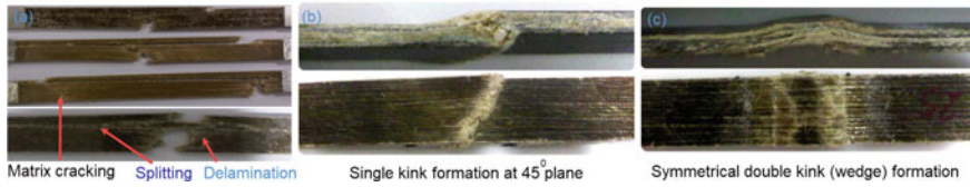
Fig. 11 Failure modes of HRFCs for a T-T, b T-C and c C-C stress ratio; reused with permission from [97]
