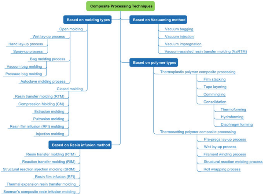
Fig. 2 Frequently used hemp fibers reinforced polymer composite fabrication techniques
