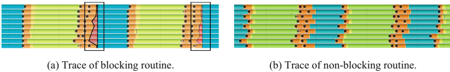
Fig. 1. Comparison of traces for blocking and non-blocking (delayed) health check routine. Computations are green and blue, communication brown, the Allreduce red.
