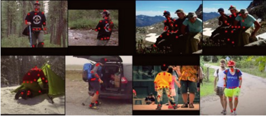
Fig. 4. Qualitative Results on MPII pose estimation result, containing viewpoint change, and occlusion and self-occlusion.
