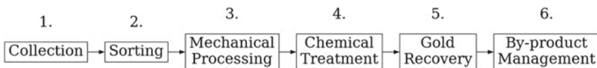
Fig. 24.2 Simplified representation of The Royal Mint's process for gold recovery from PCBs
